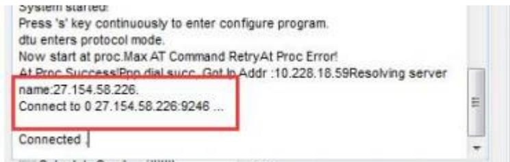
Then you can send data to test the communication between modem with data sever(here use Netassit software to simulate data server)
