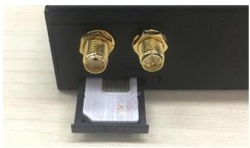
Insert the slot back to the device
