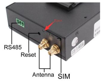
Gently press the eject button and put the SIM/UIM into the slot
